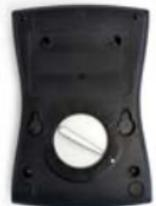
**If you do not hear an adjustable dial tone:** On the back of the hub, turn the compatibility dial very slowly until you hear a dial tone. On the front of the hub, slide the **VOLUME** adjuster until you hear a noticeable change in volume, or slide the **TONE** adjuster until you hear a noticeable change in tone quality.
