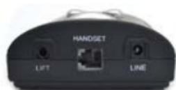
a. Remove the curly cord from the phone base, and then connect it to the **HANDSET** port on the bottom of the hub.
